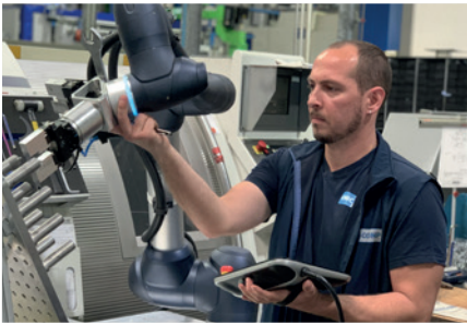
Max Schöpfer programs the robot for the CNC machine.
